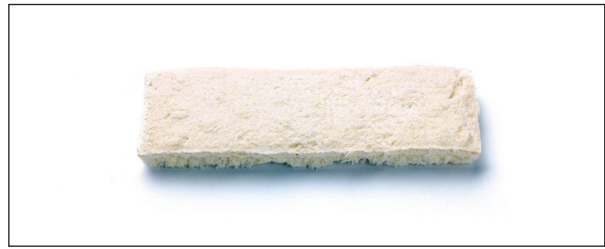
Figure 3. Composite bone substitute made of Mg-substituted HA nucleated on equine collagen fibres (type I): RegenOss®.
